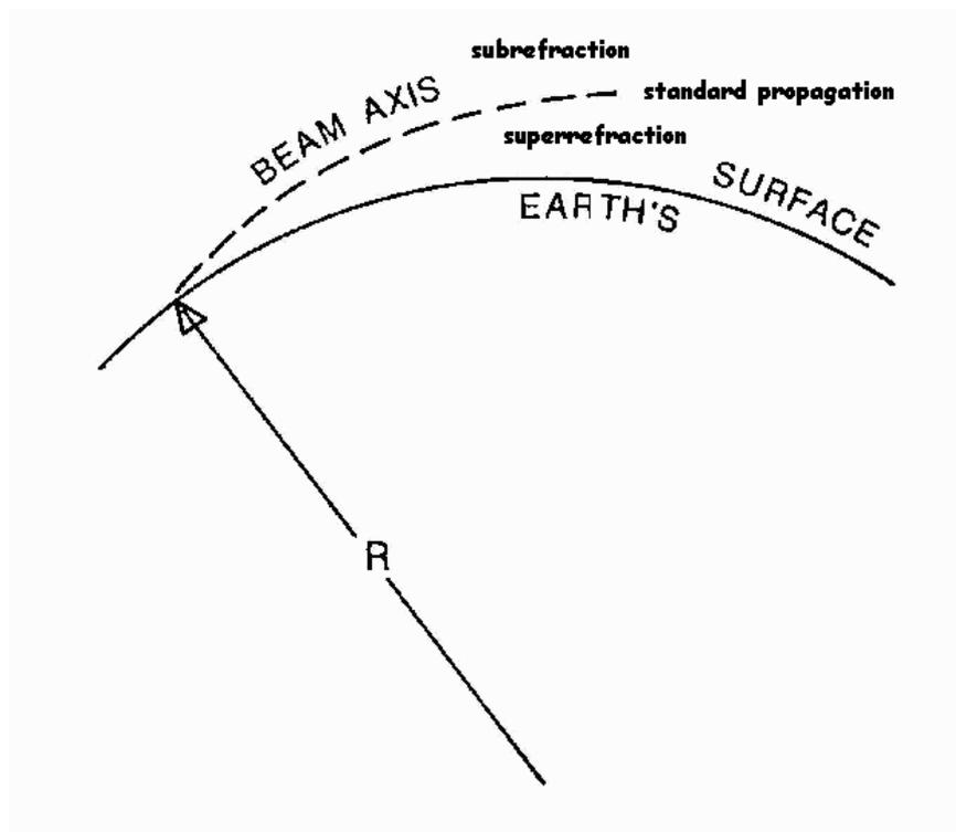
**Figure 8-4: Propagation of a radar beam.**
