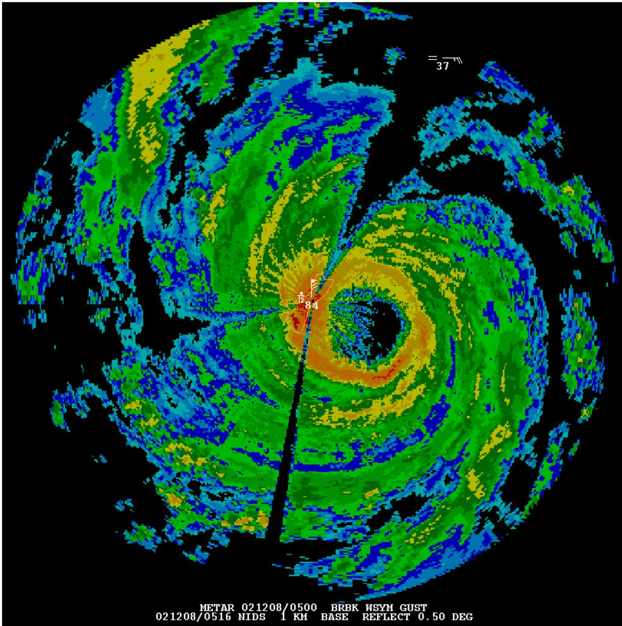
Figure 8-13: An Example of Beam Blockage (and a Typhoon)
