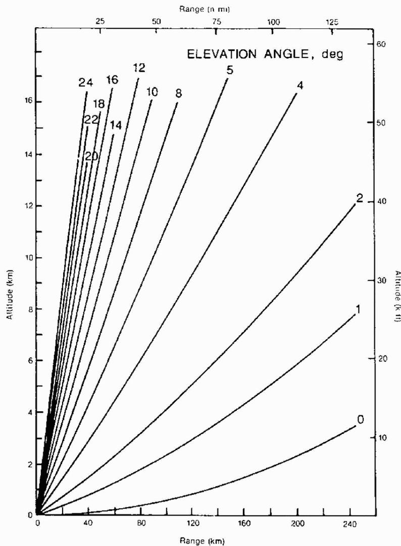
Figure 8-5: Beam height as a function of distance from the radar [source: FMH 11]
