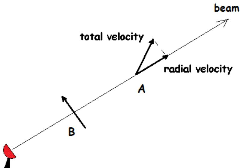
**Figure 8-6: Example of Doppler Velocity Detection**
